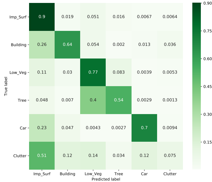
Figure 6.15: Segmentation network confusion matrix on Potsdam dataset for the considered U-net.
